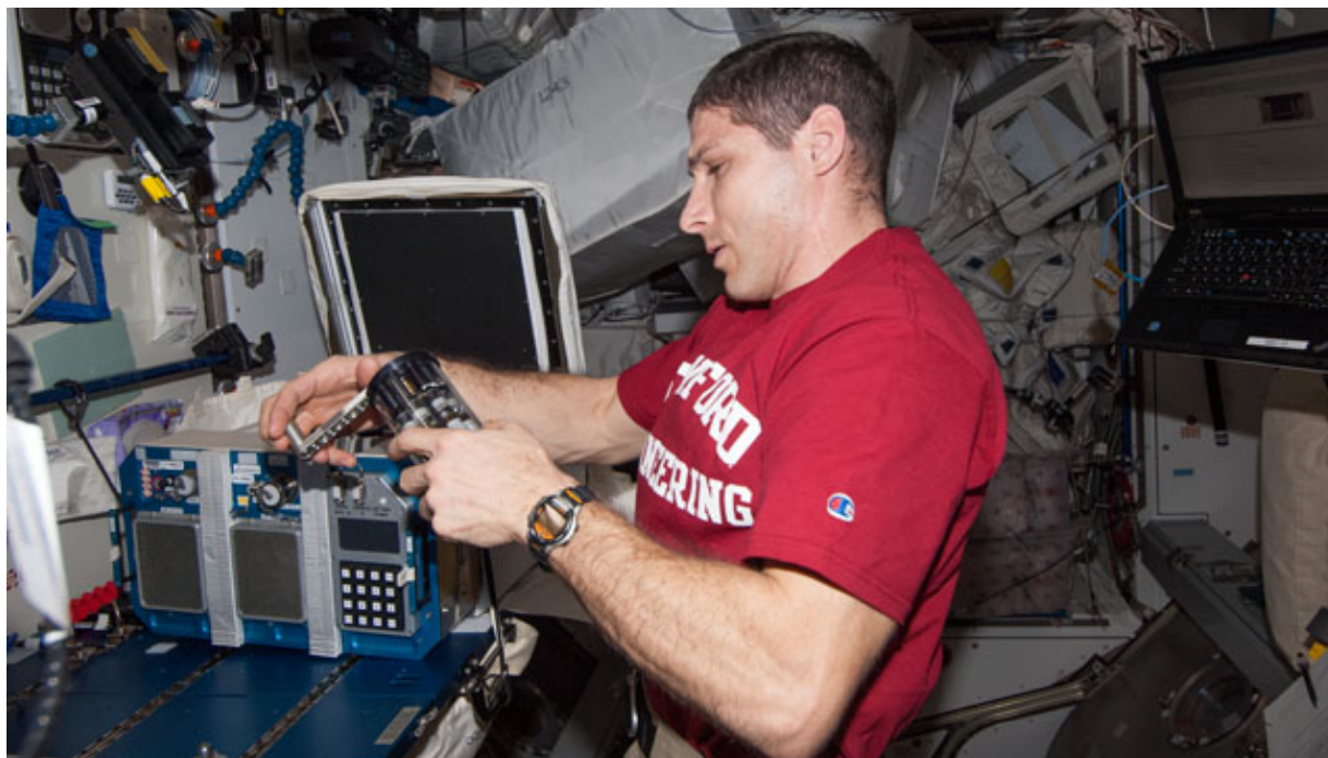
Figure 6. Astronaut Mike Hopkins operating an AES-1 GAP onboard ISS. The cranking motion allowed for the fluid in a chamber to travel to the next within each of the eight FPAs.
